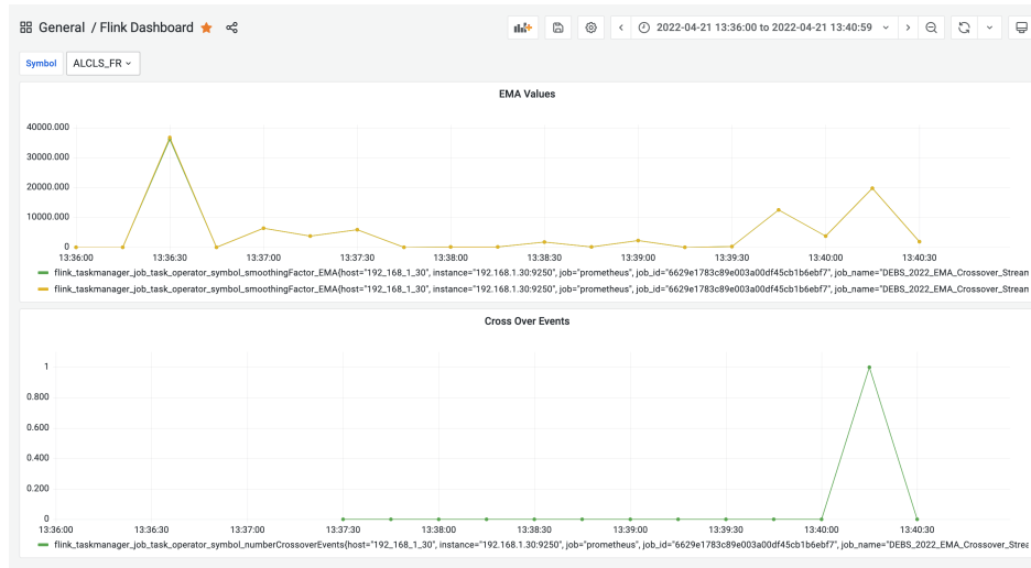
Figure 2: The Grafana dashboard showing two plots for the selected symbol ALCLS_FR. The top plot shows the EMA 38 and 100 values while the below plot shows the number of cross over events for the symbol. The legend below each plot shows the metrics from which the plot has been calculated.
